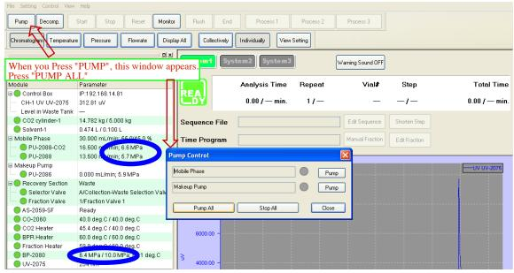
As shown below, the pressures at the two pumps rise towards ~15 MPa (150 bar) and the Back Pressure Regulator rises above 10 MPa (100 bar) and then the BPR proceeds to regulate the pressure at the 10.0 MPa setpoint selected in the Method.
