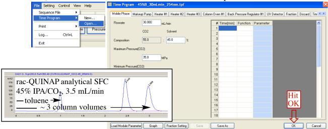
Before continuing, make sure that there is a column in the Column Oven. Also be sure that no detrimental solvents (EtOAc, CH<sub>2</sub>Cl<sub>2</sub>) remain in the system that could damage particular DAICEL columns (AD-H, OD-H).
