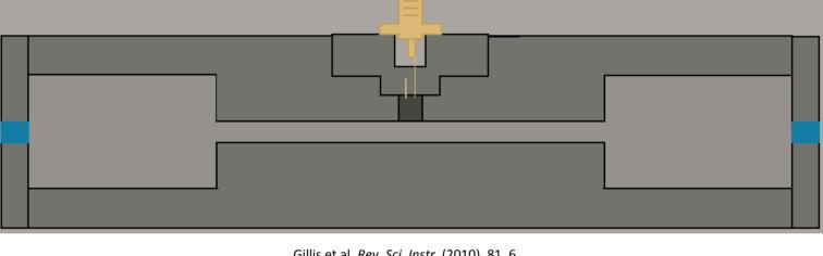
Photoacoustic absorption spectroscopy (PAS) to measure O<sub>2</sub> A-band: • Has high-sensitivity, zero-background, and large dynamic range • Tunable laser is intensity-modulated, and when laser is resonant with an O<sub>2</sub> absorption, absorbed energy is transferred to and heats the surrounding bath gas, creating a pressure wave detectable on a
