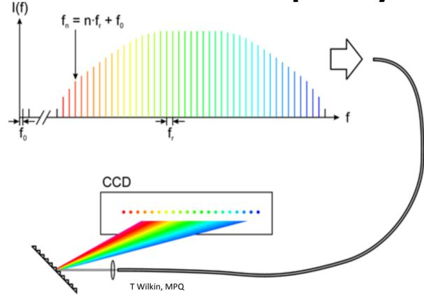
To increase the throughput and number of probe wavelengths available to study complex chemical systems, our group has begun to employ frequency comb spectroscopy. The comb spectrum is a series of equally-spaced probe frequencies, where the frequency of the  $m^{th}$  comb tooth = mf<sub>rep</sub> + f<sub>0</sub>.
