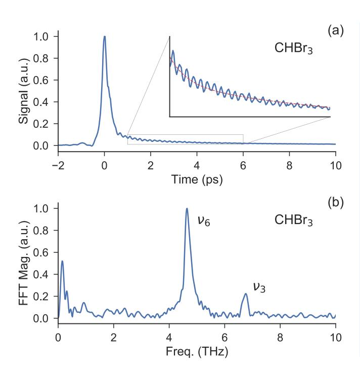
Bromoform, like many liquids, has THz-active intramolecular Single vibrational modes. shot OKE measurements (left, 50 105 (a)) are sensitive enough to detect nonlinear molecular coherences (inset). The data's FFT (b) confirms the presence bromoform's two of ot vibrational modes at 4.66 and 6.73 THz.
